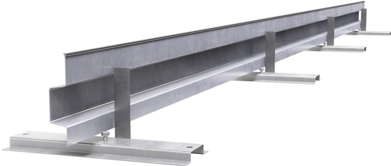
RECOSTAL® Keyboard XL units are designed for the installation of isolation joints in industrial floor slabs and deck slabs with controlled cracks along the joint. The trapezoidal profile induces a key-profiled control joint. To withstand stronger shear forces, the RECOSTAL® Keyboard XL unit can also be equipped with dowel bars. The available RECOSTAL® Keyboard XL-D variant is used to create dilatations.
